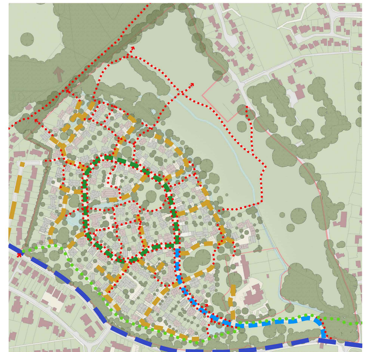
A road hierarchy with a principal road feeding into drives, lanes, and courtyards, all interlinked with a variety of paths and landscaped routes. A place that has variety and narrative.
